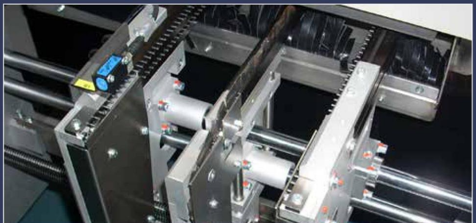
Single-lane conveyor with centre support
